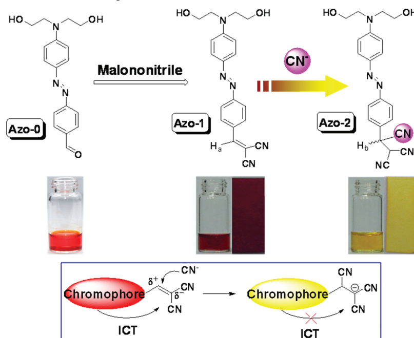
Scheme 2. Structure of Azo-1 and the Sensing Mechanism
